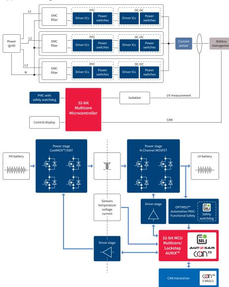
Automotive CoolSiC™ MOSFETs can either be used in the On-Board Charger (OBC, top picture showing example) application in the PFC as well as in the DC-DC stage, or in a dedicated DC-DC converter (bottom picture)
