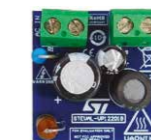
STEVAL-VP12201B 15 V/200 mA buck converter
