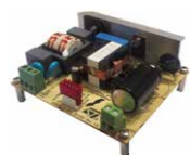
EVL6563S-100W 100 W transition-mode PFC pre-regulator
