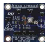
STEVAL-L7983ADJ 12 V/0.3 A step down DC/DC converter (VIN = 12 to 60 V)
