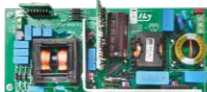
EVL6699-HVSL 150 V - 1 A LED driver featuring TM PFC and LCC resonant converter with L6699
