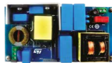
STEVAL-ILL053V2 48 V - 130 W high efficiency converter with PFC for LED street lighting
