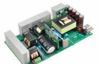
EVL400W-80PL 12 V - 400 W adapter based on CCM-PFC and HB LLC analog controller
