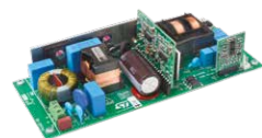
EVL150W-HVSL 150 V - 1 A LED driver featuring TM PFC and LCC resonant converter with analog combo controller
