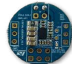
STDES-ISB38WA2 Qi-based wireless power receiver reference design for wearable applications up to 2.5 W
