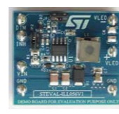
STEVAL-ILL056V1 3 A Buck LED driver board based on the LED5000
