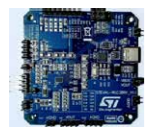
STEVAL-WLC38RX1 Qi-based wireless power receiver evaluation board for applications up to 5W BPP and 15W EPP
