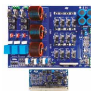
STDES-PFCBIDIR 15 kW, three-phase, three-level Active Front End (AFE) bidirectional converter
