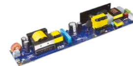
STEVAL-ILL066V2 100 W LED street lighting evaluation board with DALI2.0 communication interface using the STLUX385A digital controller
