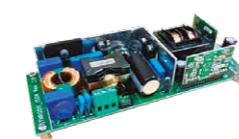
EVLSTNRG011-150 12 V - 150 W power supply based on TM PFC and HB LLC digital combo controller
