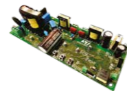
STEVAL-LLL004V1 75 W AC-DC digitally controlled non isolated constant current LED driver
