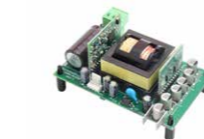
EVLMG1-250WLLC 250 W Resonant DC-DC Converter based on LLC analog controller and integrated smart GaNs
