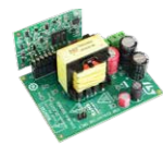
EVLIMG4-500WIBUCK High power inverse buck for dimmable LED application with GaN
