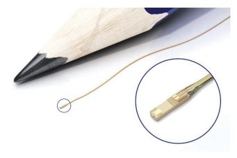
piezoresistive MEMS sensor with wire connection suitable for easy integration into invasive medical equipment.
