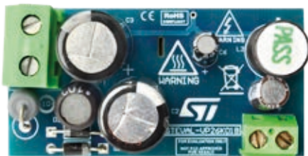
15 V / 100 mA high voltage buck converter reference design based on VIPER26K (STEVAL-VP26K01B)
