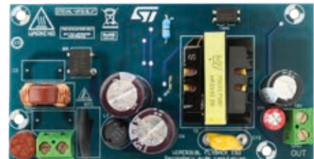
15 V / 1.2 A SSR flyback converter based on VIPer318L (STEVAL-VP318L1F)
