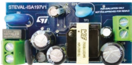
12 V, 7.8 W isolated flyback converter based on VIPer114LS (STEVAL-ISA197V1)
