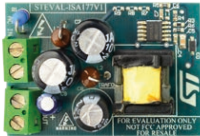
5 V / 0.85 A flyback converter evaluation board (STEVAL-ISA77V1)
