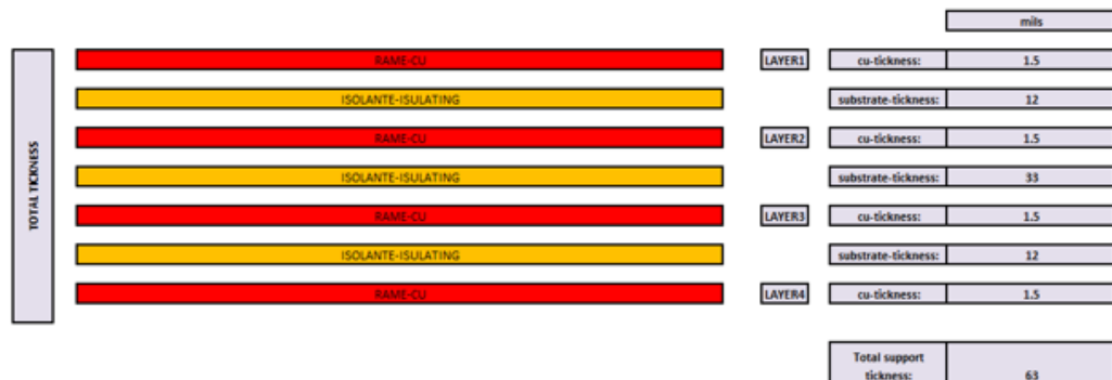
Figure 5. Four layer application board stack-up
