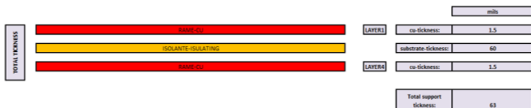
Figure 4. Two layer application board stack-up
