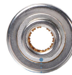
Socket in nominal position, centered relative to socket assembly outer housing
