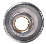
Socket position after self-aligning to the left 1.00mm relative to socket assembly outer housing
