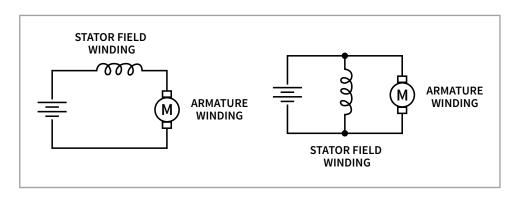
*Figure 2* Larger brushed motors use an electromagnetic field powered by the DC input. Two common arrangements are the series-wound motor (left) and the shunt-wound motor (right).
