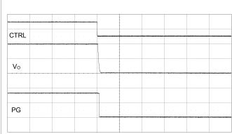
Output disabled by CTRL pin.  $V_i$  = 12 V,  $I_0$  = max  $I_0$ . Scale from top: 5, 0.5, 2 V/div, 1 ms/div.
