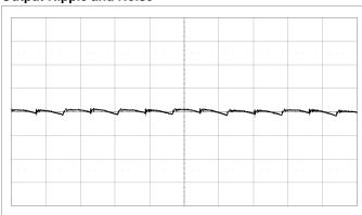
Fundamental output voltage ripple at V<sub>I</sub> = 12 V, I<sub>O</sub> = max I<sub>O</sub>, C<sub>OUT</sub> = 10 x 470  $\mu$ F/5 m $\Omega$  + 10 x 100  $\mu$ F. Scale: 10 mV/div, 2  $\mu$ s/div, 20 MHz bandwidth.
