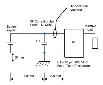
Test set-up conducted emission, power lead. DUT = Product mounted on a 182 cm<sup>2</sup> test board with the external capacitances  $C_{\text{IN}}$  = 1000  $\mu\text{F}/12~\text{m}\Omega$  + 24 x 10  $\mu\text{F}$  and  $C_{\text{OUT}}$  = 10 x 470  $\mu F/5 \ m\Omega + 10 \ x \ 100 \ \mu F$ .
