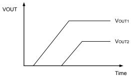
Illustration of output voltage sequencing.
