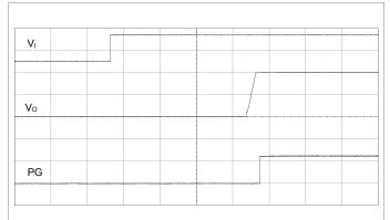
Output enabled by applying V<sub>1</sub>.  $V_1$  = 12 V,  $I_0$  = max  $I_0$ . TON\_DELAY = TON\_RISE = 5 ms, POWER\_GOOD\_DELAY = 2 ms. USER\_CONFIG = 0x1484 (PG push-pull). Scale from top: 10, 0.5, 2 V/div, 20 ms/div.
