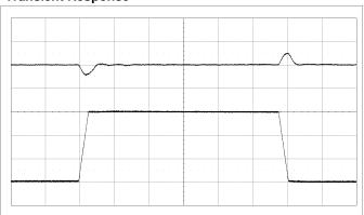
Output voltage response to load current step change (30–90–30 A) at  $V_1$  = 12 V,  $C_{OUT}$  = 10 x 470  $\mu$ F/5 m $\Omega$  + 10 x 100  $\mu$ F, di/dt = 2 A/ $\mu$ s, ASCR Gain = 300 and ASCR Residual = 90. Scale from top: 50 mV/div, 20 A/div, 100  $\mu$ s/div.
