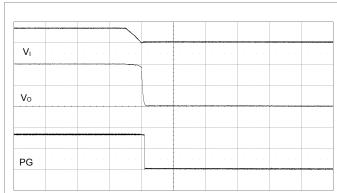
Output disabled by removing  $V_l$ .  $V_l$  = 12 V,  $I_0$  = max  $I_0$ . Scale from top: 10, 0.5, 2 V/div, 1 ms/div.
