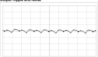
Fundamental output voltage ripple at V<sub>I</sub> = 12 V, I<sub>O</sub> = max I<sub>O</sub>, C<sub>OUT</sub> = 10 x 470  $\mu$ F/5 m $\Omega$  + 10 x 100  $\mu$ F. Scale: 10 mV/div, 2  $\mu$ s/div, 20 MHz bandwidth. See section Output Ripple and Noise.
