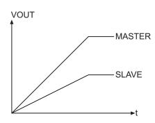
Illustration of ratiometric voltage tracking.
