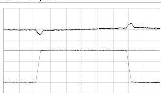
Output voltage response to load current step change (30–90–30 A) at  $V_1$  = 12 V,  $C_{OUT}$  = 10 x 470  $\mu$ F/5 m $\Omega$  + 10 x 100  $\mu$ F, di/dt = 2 A/ $\mu$ s, ASCR Gain = 300 and ASCR Residual = 90. Scale from top: 50 mV/div, 20 A/div, 100  $\mu$ s/div.
