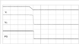
Output disabled by removing V<sub>I</sub>.  $V_I$  = 12 V,  $I_O$  = max  $I_O$ . Scale from top: 10, 0.5, 2 V/div, 1 ms/div.
