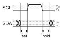
Setup and hold times timing diagram.
