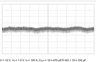
$V_1$  = 12 V,  $V_0$  = 1.0 V,  $I_0$  = 120 A,  $C_{OUT}$  = 10 x 470  $\mu$ F/5 m $\Omega$  + 10 x 100  $\mu$ F, 5 mV/div, 50 µs/div
