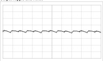
Fundamental output voltage ripple at V<sub>I</sub> = 12 V, I<sub>O</sub> = max I<sub>O</sub>, C<sub>OUT</sub> = 10 x 470  $\mu$ F/5 m $\Omega$  + 10 x 100  $\mu$ F. Scale: 10 mV/div, 2  $\mu$ s/div, 20 MHz bandwidth. See section Output Ripple and Noise.
