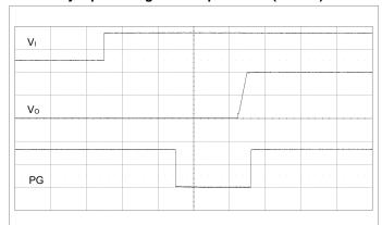
Output enabled by applying V<sub>I</sub>. V<sub>I</sub> = 12 V, I<sub>O</sub> = max I<sub>O</sub>. TON\_DELAY = TON\_RISE = 5 ms, POWER\_GOOD\_DELAY = 2 ms. USER\_CONFIG = 0x1480 (default). PG pulled up to external voltage. Note: PG being high before Vin applied can be avoided by pulling up PG to Vout. Scale from top: 10, 0.5, 2 V/div, 20 ms/div.
