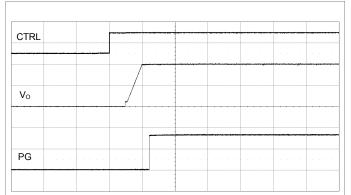
Output enabled by CTRL pin.  $V_1$  = 12 V,  $I_0$  = max  $I_0$ . TON\_DELAY = TON\_RISE = 5 ms, POWER\_GOOD\_DELAY = 2 ms. Scale from top: 5, 0.5, 2 V/div, 10 ms/div.
