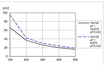
Load transient peak voltage deviation vs. ASCR gain and external capacitance. Step (30–90–30 A).
