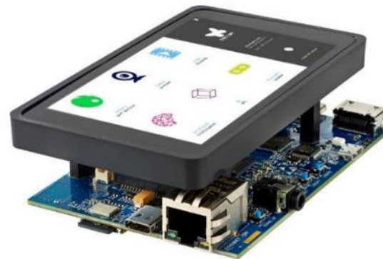
Example of STM32MP1 Discovery board used for EDGE processing
