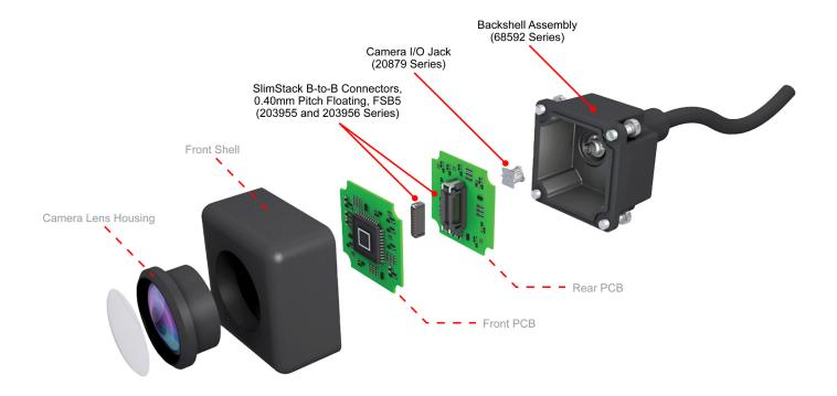
Intelligent design enables robotic assembly and meets small space requirements, critical to achieving miniaturisation in cameras, radars and LiDARs. Shown: Molex Slim Stack Floating FSB3 and FSB5 Series
