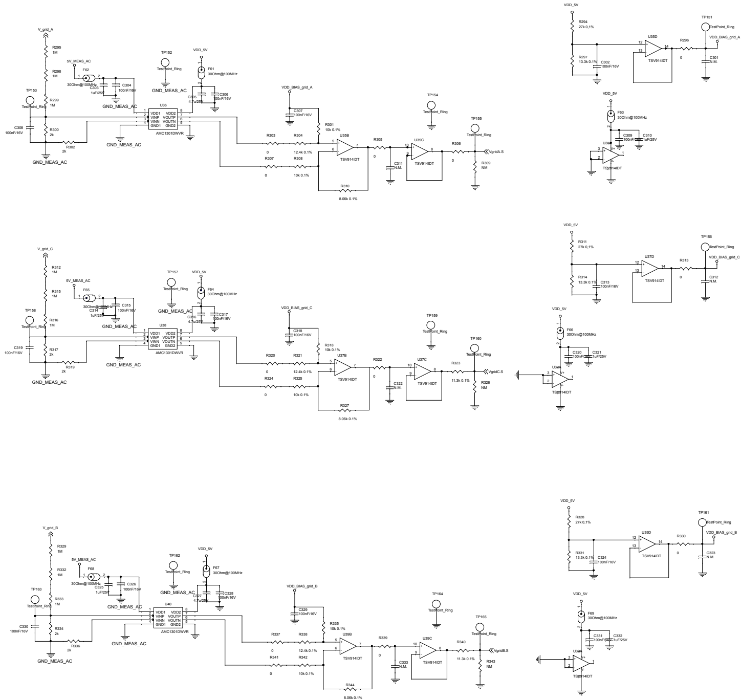
Figure 11. STDES-PFCBIDR schematic diagram - power board: grid voltage sensing
