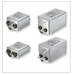
KEMET has launched a range of general purpose, single phase filters for medium to very high attenuation. The FLLE2-P, Q, R, S and U models feature a chassis mount for fast mounting, and a metal case filled with self-extinguishing resin. Fast-on or screw terminals are available, as well as options with flexible wire connections. Medical versions are available without Y-capacitors for no leakage current.
