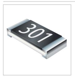
The model CMP anti-surge thick film resistor series is available in five different footprints from 0603 (1608 metric) up to 2512 (6431 metric). This product series has a wide resistance range from 10ohms to 1megohm, high rated power up to 1.5W and superior pulse load capability.
