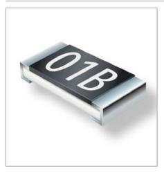
The CHP-A series sulfur-resistant, AEC-Q200 compliant thick film resistor offers triple rated power in comparison to general purpose resistors. Available in four different footprints from 0603 (1608 metric) up to 2512 (6431 metric), the CHP-A series boasts a wide resistance range from 10ohms to 1megohm, and high rated power making it ideal for current sensing and superior pulse load applications.
