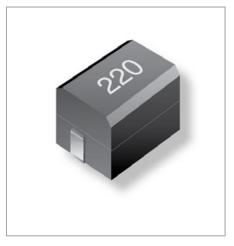
Bourns has introduced the CC322522A chip inductor series. The inductor is wound on a ferrite core which provides low DC resistance and high rated current. Encapsulation construction allows these inductors to retain high resistance to heat, humidity, mechanical shock and pressure.
