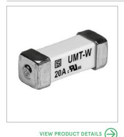
The cuboid shaped (5.3mm x 16mm), extremely compact SMD fuse is available in five rated currents from 5A to 20A and reaches rated voltages of up to 125V AC&DC with a breaking capacity of up to 1000A. Additionally, the series features a super slow and precisely defined melting characteristic unique for SMD fuses.
