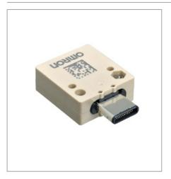
Omron Electronics XP2U test sockets are designed for testing electronic devices that have a USB type-C I/O connector. Omron XP2U sockets allow the user to connect to the testing equipment by one-touch connection to the USB Type-C connector. XP2U is ideal for testing smartphones, handheld game consoles, digital cameras, headphones, notebook computers, and more.
