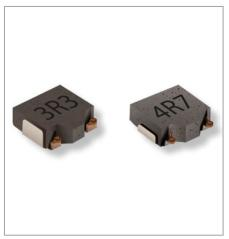
Bourns has introduced eleven high current, very low profile, shielded power inductor series designed to meet today's high current density requirement in various types of consumer electronics applications. These inductor series are manufactured with a metal alloy powder core and flat wire featuring low core loss, low DC resistance, high current, low buzz noise, excellent temperature stability and shielded construction for low magnetic radiation. Operating temperatures range from -40°C to +125°C.
