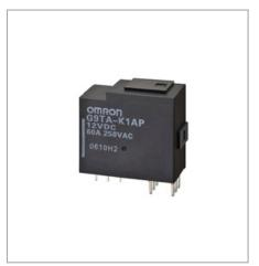
Omron has launched a PCB type version of its G9TA series AC power latching relays. Featuring a rated load of 60A and a compact size of 36.7mm x 39.1mm x 18mm, this model contributes to easy assembly in production and secure electrical connection. The G9TA series PCB type is ideal for lighting, EV chargers and inverter applications.
