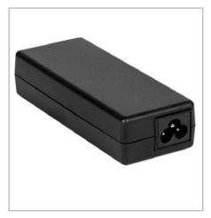
The Delta ADT-090A24AA is the newest model in the ADT series and features up to 30% reduction in size. With an efficiency up to 91.5%, the ADT-090A24AA meets efficiency DoE level VI and noload power consumption <0.15W at 115VAC and 230VAC input. The product offers a single output voltage of 24VDC with 90W output power and is suitable for general applications such as POS equipment and office equipment.
