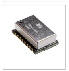
Bourns' SM41126EL LAN transformer is RoHS compliant, IEEE 802.3 Ethernet compatible, and offers a  $-40^{\circ}$ C to  $+85^{\circ}$ C temperature range. This transformer is constructed with discrete chip LAN transformers and common mode chokes assembled on a PCB with a ferrous metal shield. The SM41126EL transformer is pin-to-pin compatible with the traditional potted case LAN transformer and features a lower profile and superior coplanarity.
