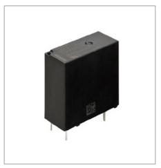
The G5PZ series of 20A power relays features a compact design with slim dimensions of  $10.5 \, \text{mm} \times 24 \, \text{mm}$  (WxL). The series features an energy saving low coil power consumption of  $530 \, \text{mW}$  in the 20A class of relays, and long life can extend end application lifetime by approximately 100,000 operations.
