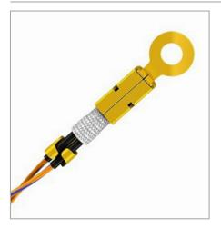
TDK has introduced the B58703M1103A\* temperature sensor which is specially developed for demanding E-mobility applications, which call for high long-term stability. The NTC sensor is designed for a temperature range of -40°C to +150°C, whereby a temporary load of up to +200°C is permitted. At +25°C the rated resistance is  $10k\Omega$  with a B25/100 value of 3625K and a tolerance of +1%.
