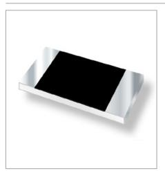
Bourns has introduced the CR01005 series thick film chip resistor. The extra small 01005 inch (0402 metric) CR01005 series broadens the general purpose thick film chip resistor family to eight different footprints up to 2512 (6431 metric).
