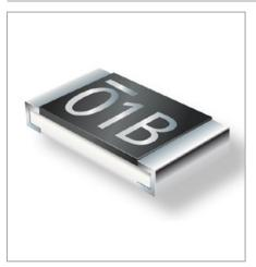
The CRxxxxA AEC-Q200 compliant chip resistor series is available in eight different footprints from 0201 (0603 metric) up to 2512 (6431 metric) and offers rated power from 0.05W to 1W. The model CRxxxxA series has a wide resistance range from 10hm to 20megohms and is designed for general purpose applications.
