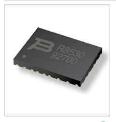
The Bourns TBU-RS085-300-WH is an integrated dual channel transient blocking, overcurrent and TVS overvoltage protector for the RS-485 communications interface. When coupled with a primary overvoltage protector like the Bourns GDT 2030-42T-SM-RPLF or TISP® Thyristor Surge Protector TISP4350J3BJR-S, the integrated solution aids compliance to IEC 61000-4-2 (ESD), IEC 61000-4-4 (EFT) and IEC 61000-4-5 (surge) standards.
