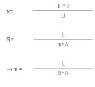
The exact value of the cell constant can be obtained as a result of calibration measurements in standard solutions. To avoid additional measurement errors, it is important to use a solution with electrical conductivity values close to the values of the intended application solution.
