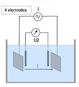
AC excitation is recommended to reduce degradation of the electrode and electrolyte.
