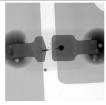
b. X-ray: fusing current of the wire bond has been exceeded
