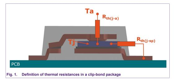
The thermal stability of a rectifier in reverse direction is determined by the interaction of its leakage current which causes self-heating, and the capability of the rectifier to dissipate this heat through the thermal resistance in the system. In thermal equilibrium, the junction temperature of the device can be described as follows with a fixed ambient temperature  $T_{amb}$  as thermal ground:
