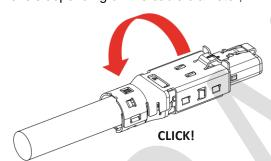
6.9 Slide the connector housing over the mounted data module until it stops. Then tighten the cable gland on block.
