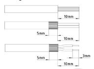
We recommend the use of a tinned copper foil to fix the braided shield.
