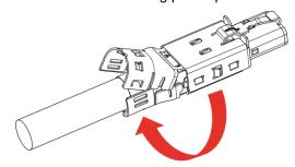
6.8 Bend the upper shielding plate downwards over the lower shielding plate until it locks with an audible "click". There are two locking levels depending on the cable diameter,
