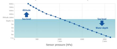
Alps Alpine's **HSPPAD143A** Pressure Sensor has an output range of 300-2100 hPa, corresponding to between around 9000 meters above sea level down to around 10 meters underwater.
