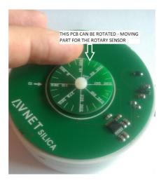
Many of the other sensors will fit on the PCB, which is located inside the module casing.
