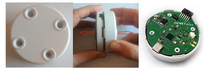
The board can run without the cover but this will lose the inductive sensor data.
