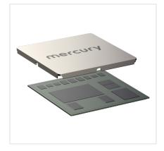
The advanced System-in-Package RFS1140 consists of an AMD Versal® FPGA, Jariet high-speed data converters and integrated power and memory. This technology, combined with Mercury's onshore design and manufacturing, brings commercial technology to mission-critical applications creating a trusted and secure solution for modern sensor processing at the edge.
