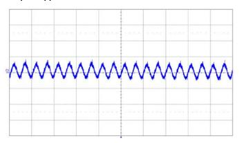
Output voltage ripple at:  $T_{P1}$ = +25°C,  $V_{I}$  = 48 V,  $I_{O}$  = 17.9 A load.
