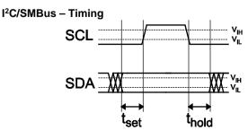
Setup and hold times timing diagram
