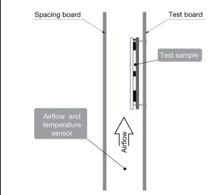
For products with base plate used in a sealed box/cold wall application, cooling is achieved mainly by conduction through the cold wall. The Output Current Derating graphs are found in the Output section for each model. The product is tested in a sealed box test set up with ambient temperatures 85°C. See Design Note 028 for further details.
