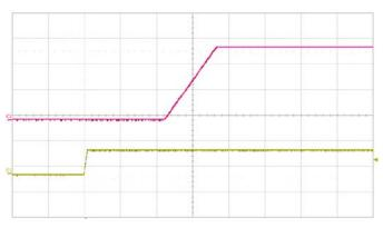
Start-up enabled by connecting V<sub>I</sub> at:  $T_{P1}$  = +25 °C, V<sub>I</sub> = 48 V,  $I_{O}$  = 17.9 A load.
