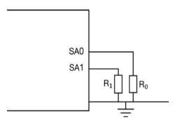
Schematic of connection of address resistors
