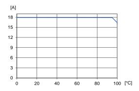
Available load current vs Base plate temperature.  $V_{\rm I}$  = 48 V. See Thermal Consideration section.
