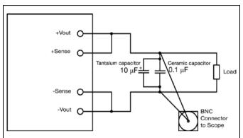
Output ripple and noise test setup
