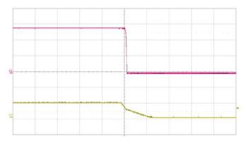
Shut-down enabled by disconnecting V<sub>I</sub> at:  $T_{P1}\!=\!+25$  °C, V<sub>I</sub> = 48 V,  $I_O$  = 17.9 A load.
