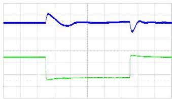
Output voltage response to load current stepchange 4.5-13.4-4.5 A (2 A/µs) at: Bottom trace: load current 5 A/div. T<sub>P1</sub>=+25 °C, VI = 48 V. with 6pcs 470µF (MPN: UPW2A471MHD) electrolytic cap
