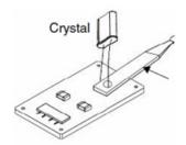
The current probe is connected to an oscilloscope and the Vp-p signal is measured. Then, using the following relationship, DL can be estimated.
