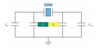
Wherein, Cin and Cout are the amplifier's input/output junction capacitances, respectively, the effective closed-loop capacitance (Ceff) seen by the crystal can be defined as:
