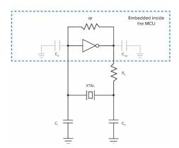
Quartz Crystals used in this approach are coined as Parallel Plated Crystals, with standard values such as 10pF, 12pF, 18pF, etc. This implies that the final oscillation frequency will be within the tolerance of the standalone quartz crystal when the closed-loop effective capacitance is <u>exactly equal</u> to the quartz plating capacitance.
