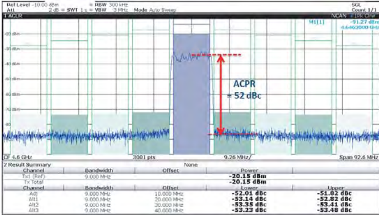
Figure 7-50. Adjacent Channel Power Ratio (ACPR) @ 6.0 GSps, 10 MHz QPSK, 4.6 GHz Center frequency, ACPR = 52 dBc, NRTZ mode
