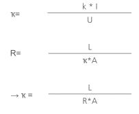
The exact value of the cell constant can be obtained as a result of calibration measurements in standard solutions. To avoid additional measurement errors, it is important to use a solution with electrical conductivity values close to the values of the intended application solution.
