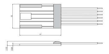
The standard IST AG LFS 117 conductivity sensor is available with either Pt/Ni wires, Ø 0.2 mm, 10 mm long or Cu/Ag wires, PTFE insulated, AWG 30.
