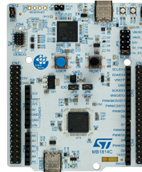
NUCLEO-H503RB NUCLEO-H533RE Affordable prototyping USB, Arduino uno IF, 64-pin MCU
