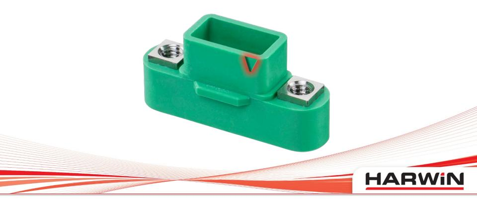
The No. 1 contact position is identified with a triangle-shaped indent on the rear wall of the crimp housings. Numbering then runs along the row, jumps back and starts again at the contact below No. 1, and runs along the second row. A 2.5mm deep potting wall is included on the housing for backpotting completed cable assemblies.
