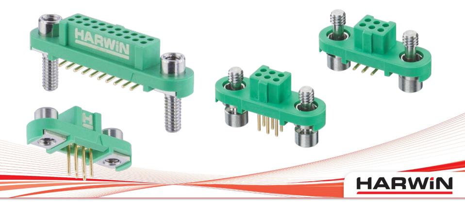
Available in <u>Throughboard and SMT</u> designs in pin counts of 6, 10, 12, 16, 20, 26, 34 and 50 contacts. The captive screws with hex socket heads prevent slipping during assembly. The design of these captive screws allows for 'Mate before Lock' – connectors can be fully mated before the screws need to be engaged. This provides for faster and easier assembly.
