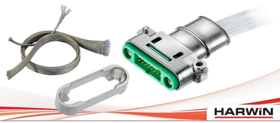
The strong and lightweight machined <u>aluminium backshells</u> provide additional strain relief. They are designed to accommodate flexible, abrasion resistant, metal braiding and are supplied with tie-bands to attach such braiding to the shell. The backshells, together with the braiding, provide shielding for enhanced electrical continuity and effective EMI/RFI protection.
