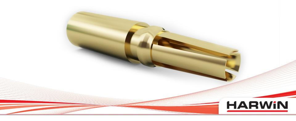
The patented single piece 4-fingered Beryllium Copper female contact gives high electrical performance and sustained mechanical durability. The crimp barrel meets IPC-A-620 specifications. It tolerates extremes of temperature, and withstands high vibration and shock. These contacts are precision-turned on state-of-the-art equipment at the UK headquarters, and plated with a gold finish to resist multiple insertions.
