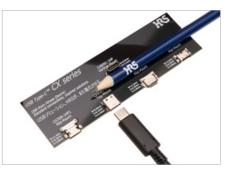
The CX series is a USB type-C 3.1 gen. 2 connector, developed as a standard high-speed transmission interface solution for consumer, industrial machinery and automotive applications. Along with various hybrid designs, and a reversible interface for easy mating, this series has a clear tactile click to ensure secure mating.
