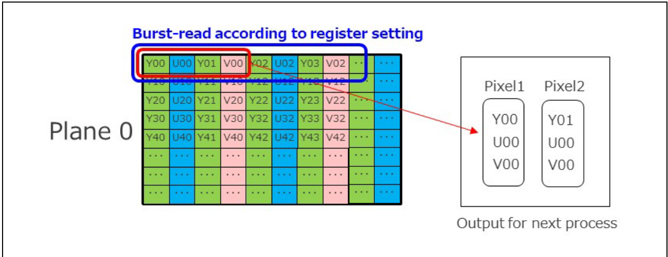
Figure 36.4 Example of Interleave Format for YCbCr422 (YUV422)
