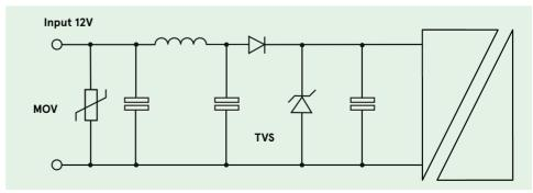
Figure 3: Automotive DC-DC input filter
