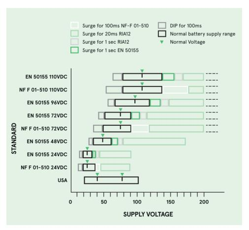
Figure 5: Input voltage ranges for rail applications
