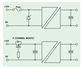
Figure 4: Reverse polarity protection options
