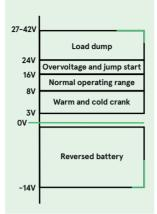
Figure 2: Summary of 12V DC-DC converter input range requirements
