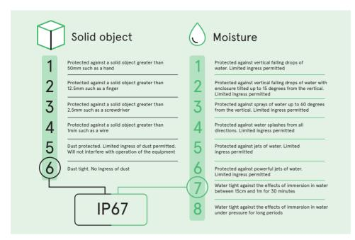
Figure 2: Ingress Protection (IP) ratings
