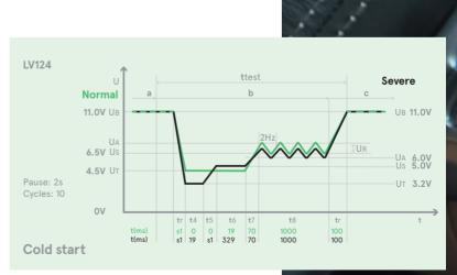
Figure 1: LV124 cold cranking conditions
