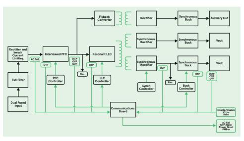
Figure 1: Typical configurable power supply architecture
