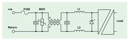
Figure 6: Common mode noise filtering
