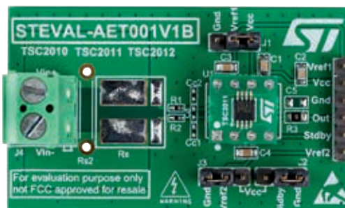
Inside the STEVAL-AETKT1V2 evaluation kit, there are one main board and three daughter boards for the TSC2010, TSC2011 and TSC2012.
