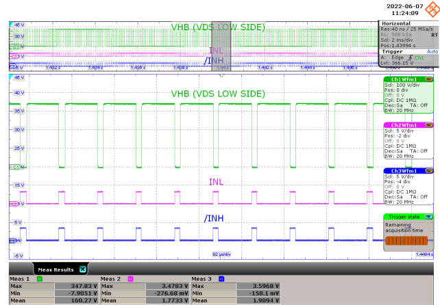
Figure 22 – INL and /INH Signal at 300 W Load.
