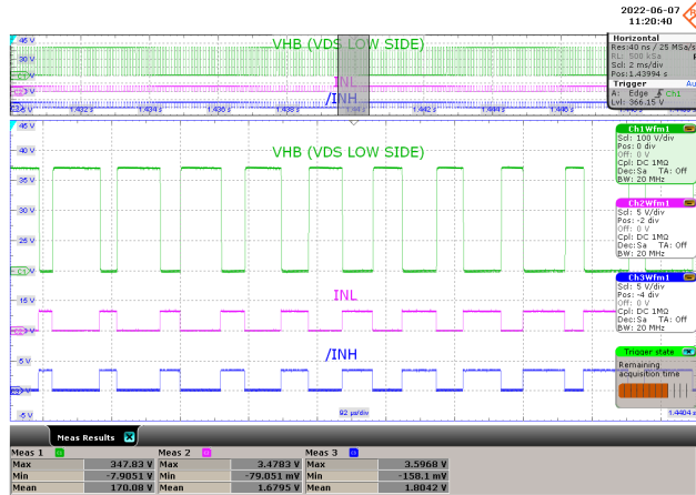
Figure 21 – INL and /INH Signal at Light Load.
