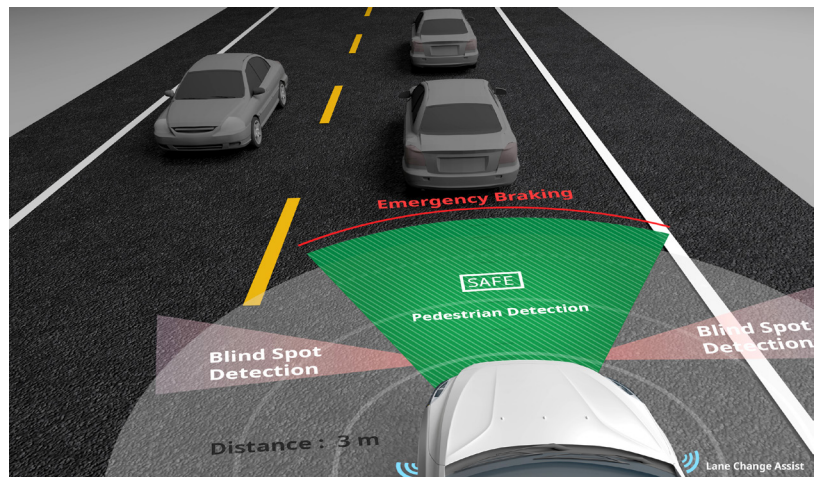
This rendering depicts just a few ADAS functionalities that combine image sensors, LiDAR and radar technologies to assess a vehicle’s true surroundings.
