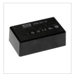
IRM-90 is a 90W miniature (87mm x 52mm x 29.5mm) AC-DC PCB-mount module type power supply, ready to be soldered onto the PCB boards of various kinds of electronic instruments or industrial automation equipments. This product allows the universal input voltage range of 80VAC to 305VAC. The 94V-0 flame retardant plastic case and the fully-potted silicone enhance the heat dissipation and meet the anti-vibration demand up to 5G; moreover, it provides the fundamental resistance to dust and moisture.
