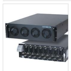
The Artesyn iHP12 configurable intelligent power system is designed to provide high accuracy, resolution and stability as a programmable voltage or current source for industrial and healthcare applications. Configurable for up to eight outputs using a wide variety of hot-swappable modules, it can provide up to 12kW in 3kW increments and address a large range of voltages and currents.
