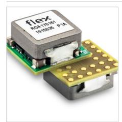
The Flex's PNA converter is an analog device with a small form factor 12mm x 12mm x 6.5mm and delivers up to 6A. The main application area is the industrial sector due to its input voltage range of 9V to 32V. The output voltage range is 0.9V to 5.5V. The PNA converter has max. power of 33W and the efficiency lies at 89.7% at 24 Vin and 3.3 Vout.
