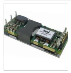
The Bel Power Solutions ORCP-D4T12x is an isolated DC-DC converter that operates from a nominal 48V source. This unit provides up to 240W of output power from a nominal 48V input. This unit is designed to be highly efficient and low cost. Features include remote ON/OFF, short circuit protection, over current protection, undervoltage lockout and over-temperature protection, pre-bias startup and power management bus. The converter is provided in an industry standard eighth brick package.
