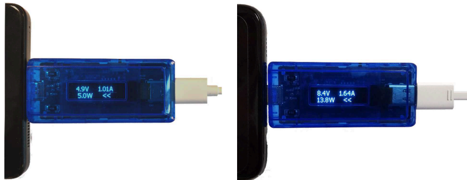
Figure 1. Charging at different V_{BUS} voltages according to the USB Power Delivery protocol
