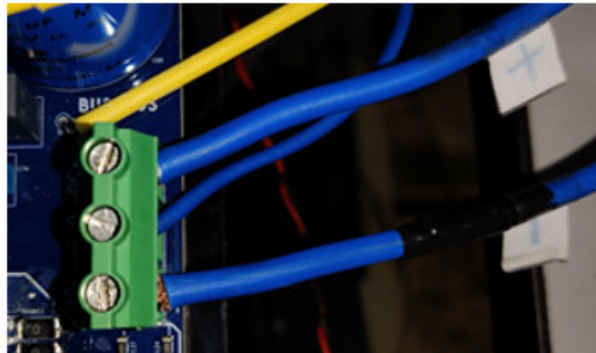
Figure 35. DC side load connection
