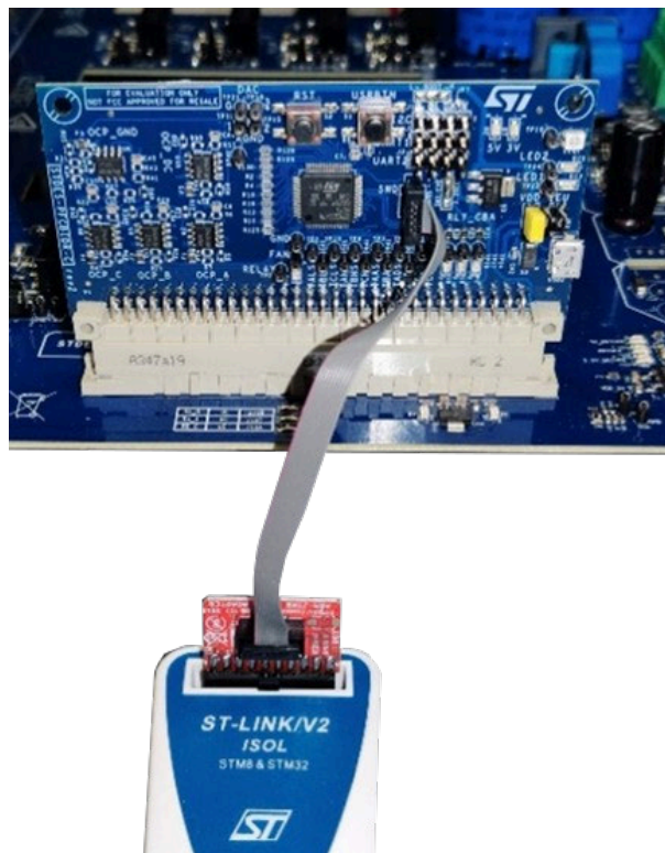
Figure 22. ST-LINK/V2 connected to the control board
