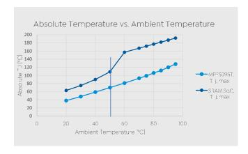
At an ambient temperature of 50°C the junction temperature of the PolarFire SoC was 70°C. The SRAM-based SoC ended up at 109°C, already beyond the industrial temperature grade which we will ignore for a moment.
