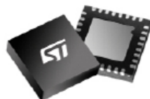
68-pin VQFN 8x8mm, 0.4mm pitch
