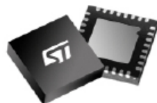
48-pin UQFN 7x7mm, 0.5mm pitch Pin-to-pin compatible
