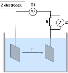
U1 = input signal (AC) U2 = output signal (AC) I = current flow R = resistor
