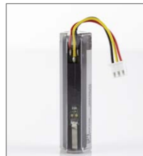
Li-Ion pack - 1S1P NCR18650 plus safety unit placed on side
