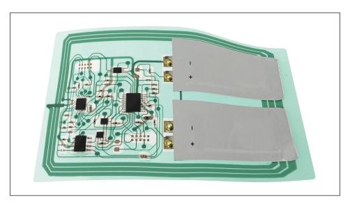
**Figure 1:** Smart labels, such as the Molex NFC Temperature Logging Smart Label, are fabricated on flexible substrates in sheet and roll-to-roll form.
