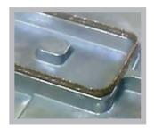
**FORM-IN-PLACE SNC45-RXP** is an Ultra-soft conductive elastomer that is dispensed onto a substrate. This soft elastomer can be dispensed into a 0.50mm wide bead. This saves space while still providing excellent shielding. The SNC45-RXP has a hardness of shore A 45 durometer. The next softest material that Laird provides has a hardness of 55. **The use of**
