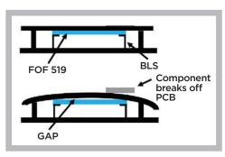
and displays) are being designed with thickness 2.00mm and below. The Ultra Soft FOF gaskets dramatically reduce the forces applied to the components compared to your standard FOF gaskets.
