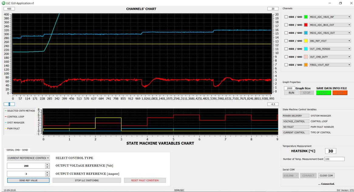
Figure 23. DC Link Voltage Increase after Defining 320 V as Set Point
