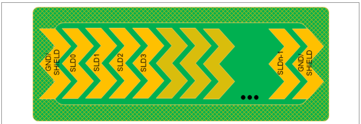
Figure 142 Linear slider pattern when first and last segments are connected to top hatch fill
