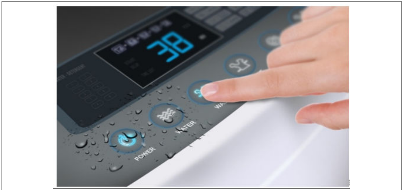
Figure 22 Liquid-tolerant CAPSENSE™-based touch user interface in washing machine
