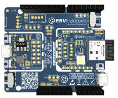
**Content:** EBV Elektronik developed a complete Software, Evaluation kit and Seminar based on Espressif ESP32-C3 & S3 Wi-Fi/BLE module with Microchip ATECC608B Secure Element, ST environmental sensors and Avnet IoTConnect cloud. Participants will benefit from our enablement software to design IoT device and cloud solutions with state of the art security, shortest time to market and most optimized cost.
