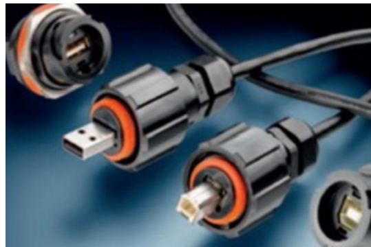
Figure 3: Circular sealed usb 2.0 connectors provide protection to IP67 thanks to their 1/4 turn bayonet coupling ring and seal.
