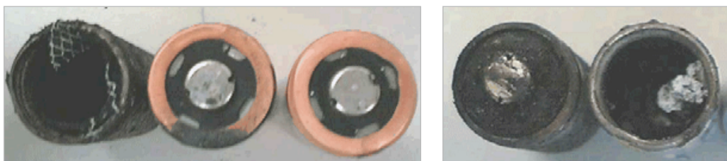
Photographic results of an in-house test with CR-123A competitor batteries (over-discharge in series)
