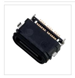
Amphenol ICC's waterproof USB Type C connectors are expected to be widely used as a next-generation interface. They support a variety of protocols such as USB 2.0, USB 3.1 Gen 1, Gen 2 and meet SuperSpeed communication 10Gb/s, 5A and 20V power supply requirements. The usability for USB 3.1 Type C connector is enhanced also by its low profile and reversible product design. Right angle stand-off, straddle mount configurations and waterproof types are available.
