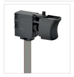
The Omron C3AW series of durable, shock resistant trigger switches from Omron is designed for DC brushless tools. The series features an anti-dust design (IEC IP6X) with a sealed cover over moveable parts and an ultrasonic welding connection between cover cases, making it ideal for cordless power tools and gardening tools.
