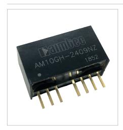
Aimtec adds the AM10G-NZ and AM10GH-NZ 10W series to its SIP8 DC-DC converter family. This new series now increases the power density of our SIP8 line from 9W to 10W. The AM10G-NZ series provides a 2:1 ultra-wide input voltage range while the AM10GH-NZ provides a 4:1 ultra-wide input voltage range (9-36VDC) and comes standard with single output voltages of 3.3, 5, 9, 12, 15 and 24VDC with I/O isolation of 1500VDC.
