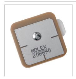
The Molex GNSS/GPS-enabled devices need highly compact antennas with high radiation efficiency performance. Measuring only  $3.20 \times 1.60 \times 1.10$ mm, Molex low-profile GNSS ceramic antennas offer maximum space savings with an average total radiation efficiency of at least 60% over 1561 to 1602MHz bands.
