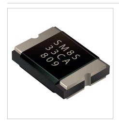
The Bourse SM8SF-Q series is AEC-Q101 compliant and well suited for protecting sensitive electronics against voltage transients generated by inductive load switching and lighting. Bourns® model SM8SF-Q series offers a high Peak Pulse Power (PPK 10/1000µs) of 7000W, assisting designers in meeting ISO7637-2/ISO16750-2 surge specifications. This AEC-Q101 compliant product is also well suited for applications requiring high reliability such as power supplies and equipment used in harsh environments.
