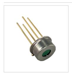
TE Connectivity introduces the Digital Thermopile Sensor (TSD) contactless temperature measurement system which addresses a full range of critical design and performance demands: accuracy, speed, low power/energy efficiency, and limited space requirements. The TSD sensors include an infrared sensor (thermopile) and a sensor signal conditioner, and can be interfaced to any microcontroller by an I2C interface.
