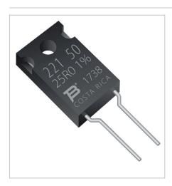
Bourns is pleased to announce the introduction of the new model PWR221T-50 series high power thick film resistors. This series is available in a compact TO-220 package utilising thick film on ceramic technology which provides the advantage of low inductance and the ability to absorb power up to 50 watts when properly mounted to a heat sink.
