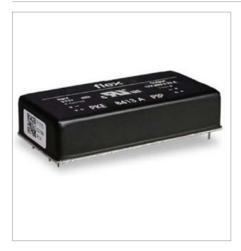
Flex Power Modules was pleased to introduce the PKE-A series of DC-DC power modules for the industrial and railways sectors, broadening its product range to meet increasing demand in these sectors. The modules are provided in sealed and encapsulated packaging, to ensure they will work reliably when subjected to dust, moisture, severe vibration and other harsh conditions.
