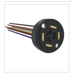
The Amphenol ICC FLA series dimming receptacle - ANSI C136-41 is designed with power and dimming/signal contacts to provide a connection between dimmable photocell and the luminaire for commercial and utility lighting.
