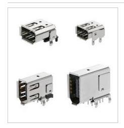
Molex's 2.00mm I/O connector system is available in 6, 8 and 10 circuit options. The 6 and 10 circuit connector systems feature auto-mounting and reflow-soldering for wire-to-wire applications. Additionally, the 6 circuit option conforms to the IEEE 1394 standard, making this system ideal for industrial control applications.
