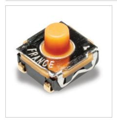
The C&K KSC DCT series offers sealed tactile switches for SMT with SPDT function. This dual-circuit functionality provides two outputs from a single input. Housed in a tiny 6.2mm x 6.2mm x 2.9mm PCB-mount package, the silicone 70SH actuator included in the package extends the height to 5.2mm above the PCB surface for easy operation and easier integration through pre/post travel.
