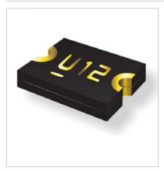
The Bourns Multifuse product line was pleased to introduce the 12V rated model MF-USML/X series of low resistance surface mount Polymer Positive Temperature Coefficient (PPTC) resettable fuses. The series includes Ihold current ratings from 1.75A to 5.5A at the 12V maximum rated voltage.
