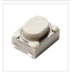
The C&K PTS815 series offers tactile switches with a 4.2mm x 3.2mm footprint in SMT version with 2.5mm height. Three actuation forces are available: 180gf, 250gf and 400gf. Its hard actuator ensures that it can be integrated into standard processes, with no need for an additional interface button. These small tactile switches have an operating life lasting up to 100,000 actuations.
