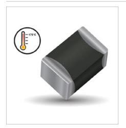
The AVX TransGuard® VT series high-temperature MLVs provide extremely reliable bidirectional overvoltage protection across operating temperatures extending from -55°C to +175°C with zero derating across the entire range, are qualified to AEC-Q200, and are currently available in compact, surface-mount 0603 and 0805 cases sizes.
