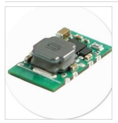
The Aimtec AMSRL-Z switching regulator is an ultra-low-profile open frame non-isolated DC-DC converter. The dimensions of AMSRL-Z series are of 19.5mm x 11.8mm x 5mm which is extremely compact for this class.
