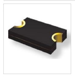
Bourns Multifuse product line was pleased to introduce the 8V and 6V rated model MF-FSML/X series of low resistance surface mount Polymer Positive Temperature Coefficient (PPTC) resettable fuses. The series includes Ihold current ratings from 0.35A to 1.75A at the 8V maximum rated voltage, and Ihold current ratings from 2A to 3A at the 6V maximum rated voltage.
