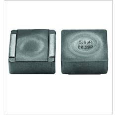
Vishay was pleased to introduce an automotive grade IHLP low profile, high current inductor in the 6767 case size. To save space in under the hood automotive applications, the Vishay Dale IHLP-6767GZ-8A combines a high continuous operating temperature to 180°C with a low profile of 7mm.
