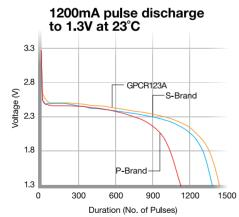
**Excellent Pulse Discharge Performance at Room Temperature** GPCR123A shows superior high pulse discharge performance and longer duration than competitors.
