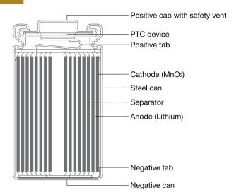
GP Primary Lithium 9V battery (GPCR-V9) is consisted of 3 pieces of GP Primary Lithium Cylindrical Batteries (GPCR14250)
