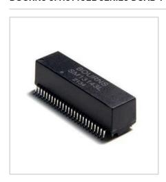
Bourns is introducing the new Model SM13143EL Dual-Port LAN 10/100/1000 Base-T PoE++ transformer for Ethernet applications. This LAN transformer is IEEE 802.3bt Type 3 4PPoE compliant and PoE++ capable of up to 60W with 700mA DC balance current to support each channel, or 1400mA DC balance current to support full channels. The transformer's operating temperature range is from -0°C to +70°C with 1.5kVrms isolation voltage.
