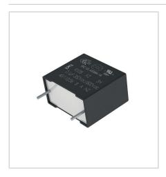
The R53B series is constructed of metallized polypropylene film encapsulated with selfextinguishing resin in a box of material that meets the requirements of UL 94V-0. The R53B series is ideal for harsh environmental conditions and meets the demanding automotive electronics council's AEC-Q200 qualification requirements.
