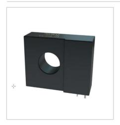
The FG-R05-4A sensor is a high-sensitivity AC and DC leakage current sensor with individual open drain alarms and an analog output for leakage current indication. In addition, its integrated test coil can be initiated by a test input to perform a functional alarm test.
