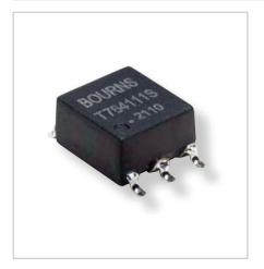
The Bourns is introducing the new model PAD00x-T764 push-pull isolation transformer deries. The model PAD00x-T764 series are low profile, small footprint isolation transformers, with a primary inductance of  $475\mu H$ , maximum  $11V-\mu S$ , 400VDC continuous operation, low DC resistance of  $550m\Omega-800m\Omega$  maximum, and an operating temperature range of  $-40^{\circ}C$  to  $+125^{\circ}C$ .
