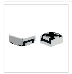
Vishay/Dale IHLE® high current inductors are AEC-Q200 qualified devices with integrated e-field shields that negate the need for separate shielding. The IHLE series is rated for temperatures up to +155°C. These inductors offer excellent DC-DC energy storage up to 2MHz and 20dB e-field reduction at 1cm. Vishay/Dale IHLE® High Current Inductors withstand high transient current spikes without saturation.
