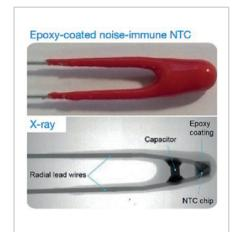
With increasing complexity of electric systems and density of electronic components in modern vehicles, conventional NTC thermistor sensors are vulnerable to stray electromagnetic interference causing self-heating.
