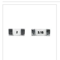
Eaton Bussmann Series 1145HV & 1350HV fast-acting fuses provide reliable overcurrent protection up to 5A for high voltage applications. Both product families are available in surface mount printed circuit board packages with the 1145HV in 11mm x 4.5mm footprint and 1350HV in 13mm x 5mm footprint. The high voltage ratings and SMD package help reduce required PCB space.
