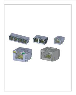
The RJE3A series of modular jacks is a SMT connector that meets CAT5e performance per EIA-568-C.2. It supports gigabit ethernet protocols as well as 2.5GBASE-T per IEEE 802.3bz. Shielding available for improved EMI performance and LEDs for link activity and network speed verification.
