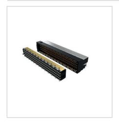
The BergStak® secure connector family contains one-time-use and multi-times-use solutions to support customers different needs on connection security. The family now contains variants with 3-row and 4-row contacts with 37 columns per row, and it can be extended in both (10) row and (100) column direction based on customer requirements, to fulfill high pin count/high signal density requirements.
