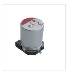
KEMET's surface mount solid polymer aluminum capacitors offer longer life and greater stability across a wide range of temperatures. This highly conductive solid polymer electrolyte eliminates the risk of drying out and, due to its low ESR properties, is able to withstand higher ripple currents during normal operation. This series is ideally suited for industrial and commercial applications.
