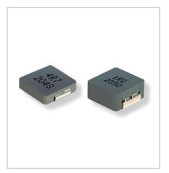
Bourns is introducing the new automotive grade Model SRP7020TA and SRP8540A series high current shielded power Inductors that have been designed to meet today's high current density and high temperature requirements of various electronic applications. These inductor series are manufactured with a metal alloy powder core featuring low DC resistance, high heating/saturation current, low buzz noise, excellent temperature stability and shielded construction for low magnetic field radiation.
