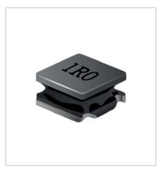
Effective immediately, Bourns magnetics product line is introducing the new model SRN3015C series Semi-shielded power inductor. Constructed with a magnetic-silica coating to the perimeter of the inductor winding to provide effective shielding, these inductors release lower magnetic field radiation compared to non-shielded inductors. These new semi-shielded inductors are lower priced than typical comparably-sized conventional ferrite shielded inductors.
