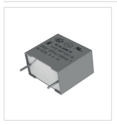
The R41B is constructed of metallized polypropylene film, encapsulated with self-extinguishing resin, in a box of material meeting the requirements of UL 94V-0. automotive grade devices meet the demanding automotive electronics council's AEC-Q200 qualification requirements.
