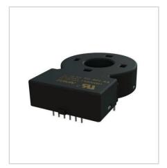
The FG-R01-4A sensor is a high-sensitivity AC and DC leakage current sensor with individual open drain alarms and an analog output for leakage current indication. In addition, its integrated test coil can be initiated by a test input to perform a functional alarm test.
