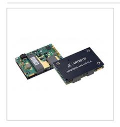
ADQ600B series quarter-brick isolated DC-DC converters produce a single fully regulated 12V output. Rated at 600W, these converters can deliver up to 50A output current and have no minimum load requirement. They have an input voltage range of 36V to 75V and are primarily designed for use with standard 48V supplies in computing and server applications, as well as regulated 48V supplies in communications equipment.
