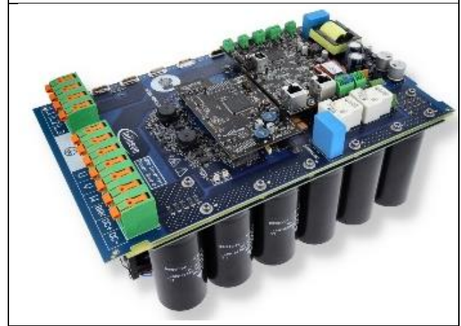
Fig. 2 Drives inverter for testing two-level slew-rate control
