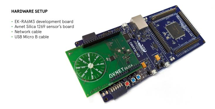
Plug the 1269 board into the EK-RA6M3's Arduino shield.
